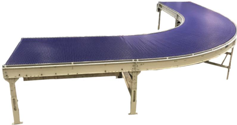
Systec's Stable Stack Bundle Conveyor (SSBC) is a material handling solution for applications in which a smooth surface is required. The SSBC Curve has advantages over standard bundle conveyor curves because it eliminates the gap between rollers and product maintains a 90 degree orientation.
