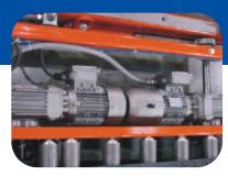
DRIVE ASSEMBLY Systec's transfer car drive assemblies operate the conveyors and side shifting beds. The car features a fixed or variable speed, five horsepower gearmotor for
