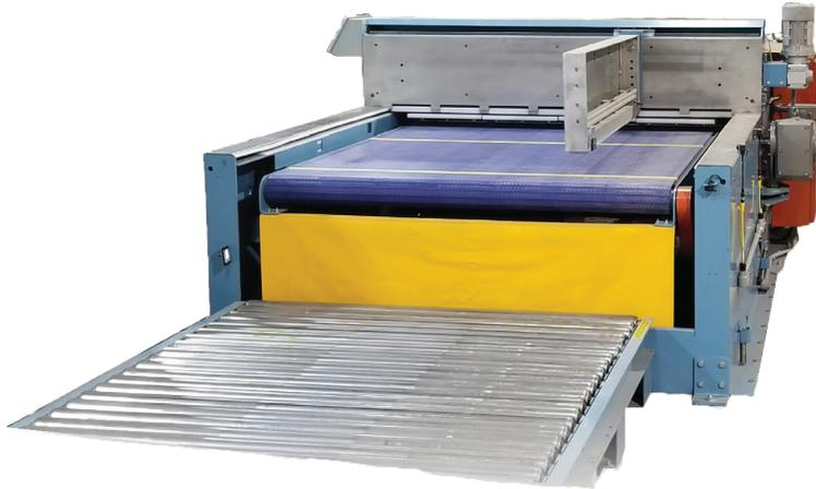
Systec's redesigned Load Former is an exceptional machine for ergonomic unit-load building. Operators can move bundles without lifting to build tiers to the finished unit-load.
