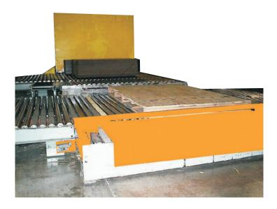
Systec's Pallet Sweep Device (PSD) is an efficient way to remove corrugated loads off of pallets to infeed a machine.
