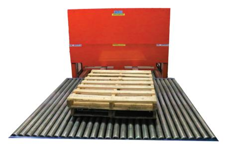
Systec's Pallet Handling Device (PHD) is a safe and efficient method of dispensing pallets.
