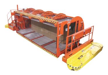
Systec's Load Inverting Device (LID) will enhance your efficiency of corrugate inversion for botton side printing applications.
