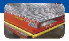
**OVERALL CONSTRUCTION** Systec's SPC features welded steel frame construction with precision laser cut parts. This is a self-contained unit.
