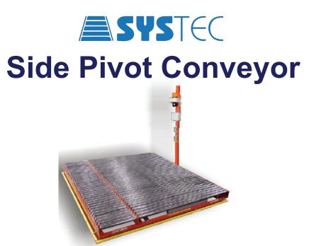
Systec's Side Pivot Conveyor (SPC) can be used at various points within the overall conveyor system. The SPC is primarily used where change in load direction is required, yet the load orientation must remain the same. This is particularly applicable where pallets may be used within the system. This is due to the fact that the pallet's runners, or bottom boards, must remain perpendicular to the load carrying rollers to smoothly convey the load.
