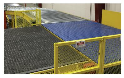
Performance Line Passive Right Hand Transfer (PRAT)Systec's Performance Line Passive Right Angle Transfer or PLRAT is designed to allow for instantaneous transitions of loads, all while maintaining orientation. It is an alternative to belt transfers and allows for more flexibility and load building capabilities, all while maintaining a smaller foot print than a traditional 90° degree curve.
