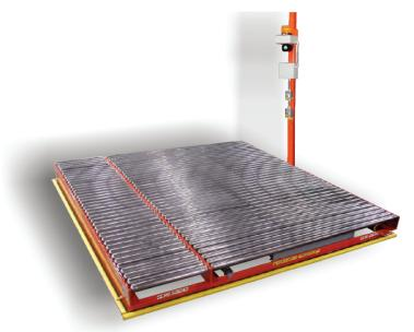
Systec's Shuttle Automatic Car (SAC) can be used at various points within the overall conveyor system. The SAC is primarily used where a break in the conveyor line is required, or a single line may need to deliver to more than one location. It can also be used at the infeed of converting equipment to allow machine opening without interference.
