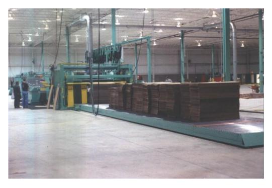
Systec's Mobile Infeed Conveyor (MIC) is designed for converting machine infeed, and can move with the "roll-out" for maintenance and change-out. The MIC can be a self-contained power driven unit, or it can be attached to the converting machine feed table for in/out movement. It can be designed for automatic prefeed, or it can be equipped with a lift table for manual operator feed systems. Systec's MIC is a solid replacement for existing shuttle cars.
