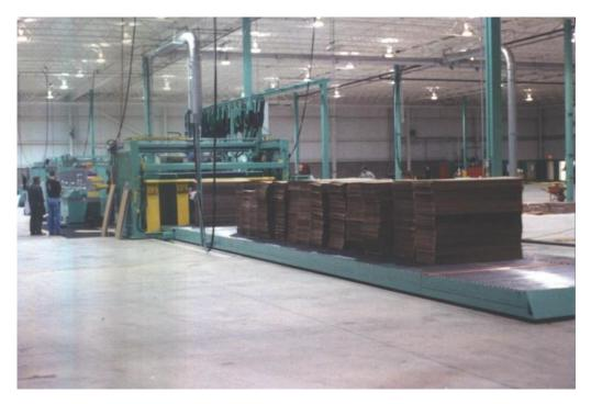
Systec's Mobile Infeed Conveyor (MIC) is designed for converting machine infeed and can move with the "roll-out" for maintenance and change-out. The MIC can be self-Contained power driven or it can be attached to the converting machine feed table for in/out movement. It can be designed for automatic prefeed, or it can be equipped with a lift table for manual operator feed systems. Systec's MIC is a solid replacement for existing shuttle cars.
