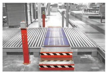
Systec's Conveyor Safe Walk (CSW) is a safe and efficient method of creating safe passage across any conveyor mainline. Our newest version has been completely redesigned to increase the drive consistency and overall durability of the CSW. This redesign makes Systec's CSW the longest lasting plastic conveyor crossing design in the industry.
