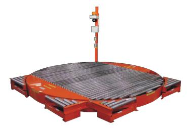
Systec's Center Pivot Conveyor (CPC) can be used at any point within the overall conveyor system. The CPC is primarily used where change in load direction is required, yet the load orientation must remain the same. This is particularly applicable where pallets may be used within the system. This is due to the fact pallets runners, or bottom boards, must remain perpendicular to the load carrying rollers to smoothly convey the load.
